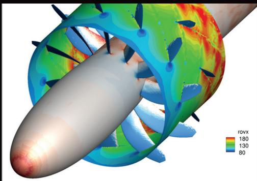
Large-Eddy simulation of a counter rotating open rotor. © ISAE-SUPAERO
