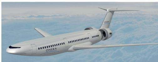
Configuration with boundary layer ingestion. © ONERA
