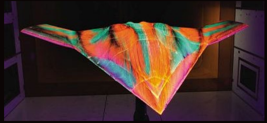
Aerodynamic visualization in wind tunnel on a fighter aircraft - Credit ONERA
