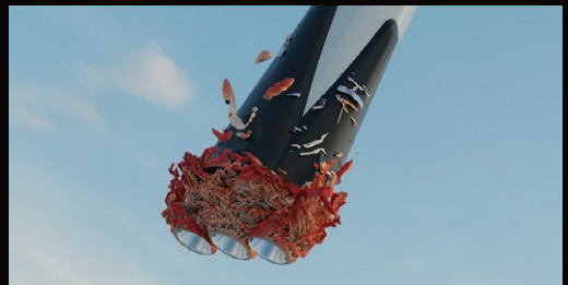
LES computation on a future reusable launcher configuration with 3 nozzles - Credit ArianeGroup
