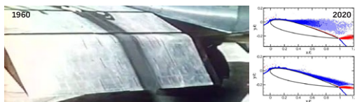
Active flow separation control on NACA airfoil, PIV measurements, 2020 Credit PPRIME
