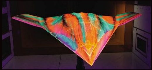
Aerodynamic visualization in wind tunnel on a fighter aircraft - Credit ONERA
