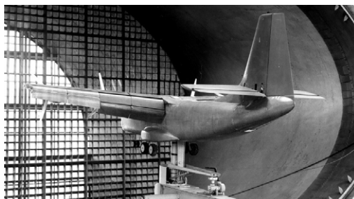
Chalais-Meudon tests of flow separation control Bréguet Vultur, H. Poisson-Quinton, 1960 - Credit ONERA
