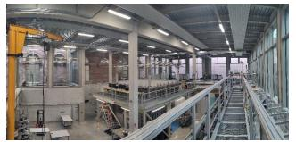
The MechaniCS platform brings together all the pilots and experiments relating to mechanics research at the ICube laboratory, as well as the expertise of the staff working there. The mechanics of materials platform brings together devices for characterising static/quasi-static materials at medium and high speeds. It includes two high- and low-elongation test machines. It also includes several drop towers for characterising materials and structures under impact.
